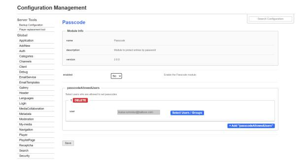
The **Module Info** box displays the module name, description (what enabling this module allows users to do), and version number.
