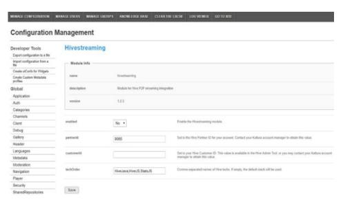
The Module Info box displays the module name, a description of the module (what enabling this module allows users to do), and a version number.
