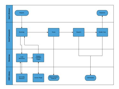
Most of the flow actually represents processes that are managed by the Zend Framework (such as bootstrap and dispatch). The interesting and important part of the diagram is the bottom swim lane – controlled by the KMS Library. These are the main entry points where KMS interacts with modules.
